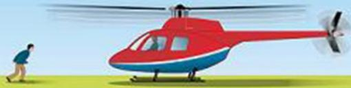
Do not approach without receiving a visual signal from the pilot. Do not leave without a visual or spoken instruction to do so. Stay where the pilot can see you at all times.
