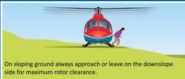
On sloping ground always approach or leave on the downslope side for maximum rotor clearance.
