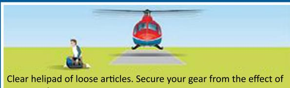
Clear helipad of loose articles. Secure your gear from the effect of rotor wash.
